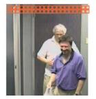
After inverting the mask: the movement of personnel in front of the door is ignored; only door movements are detected.
